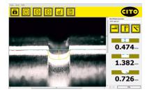
CITO CounterControl is an optical, non-contact measurement system for monitoring the width and depth of the creasing channel in Pertinax and the counter plate.
